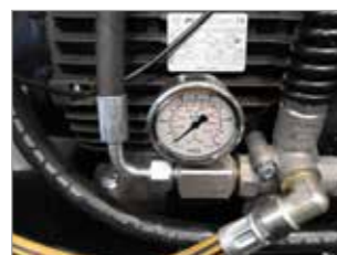
PROFESSIONAL PRESSURE GAUGE ENABLING THE CONSTANT MONITORING OF WORKING PRESSURE
