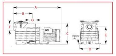
These self priming centrifugal swimming pool pumps feature injection moulded glass reinforced thermoplastic body and strainer, with Noryl impeller and stainless steel inserts and fixings. The pre-filter section has a drain plug, transparent polycarbonate screw-down lid with O-ring seal and injection moulded white filter basket.
